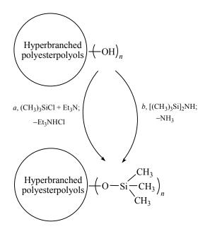
The products are highly viscous fluid resin soluble in organic solvents like acetone, chloroform, diethyl ether. The modification of the initial hyperbranched polyesterpolyols by the introduction of trimethylsilyl fragments led to an increase in fluidity and hydrophobicity of the polymer.
